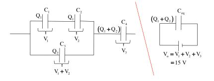
$C_{1}=15 \ \mu F$   $C_{2}=3 \ \mu F$   $C_{4}=20 \ \mu F$   $C_{6q}=5.96 \$
