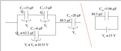
So if we were masochists, we could start with  $V_1+V_2=10.53~V$ , note that  $V=\frac{Q}{C}$ , and solve for the Q's . . . or we could be clever and note that if  $\left(Q_1+Q_2\right)=89.5~\mu F$ , and if, as we've deduced,  $Q_2=63.2~\mu C$ , then  $Q_1$  must be  $26.3~\mu C$ . QED (hee, hee).
